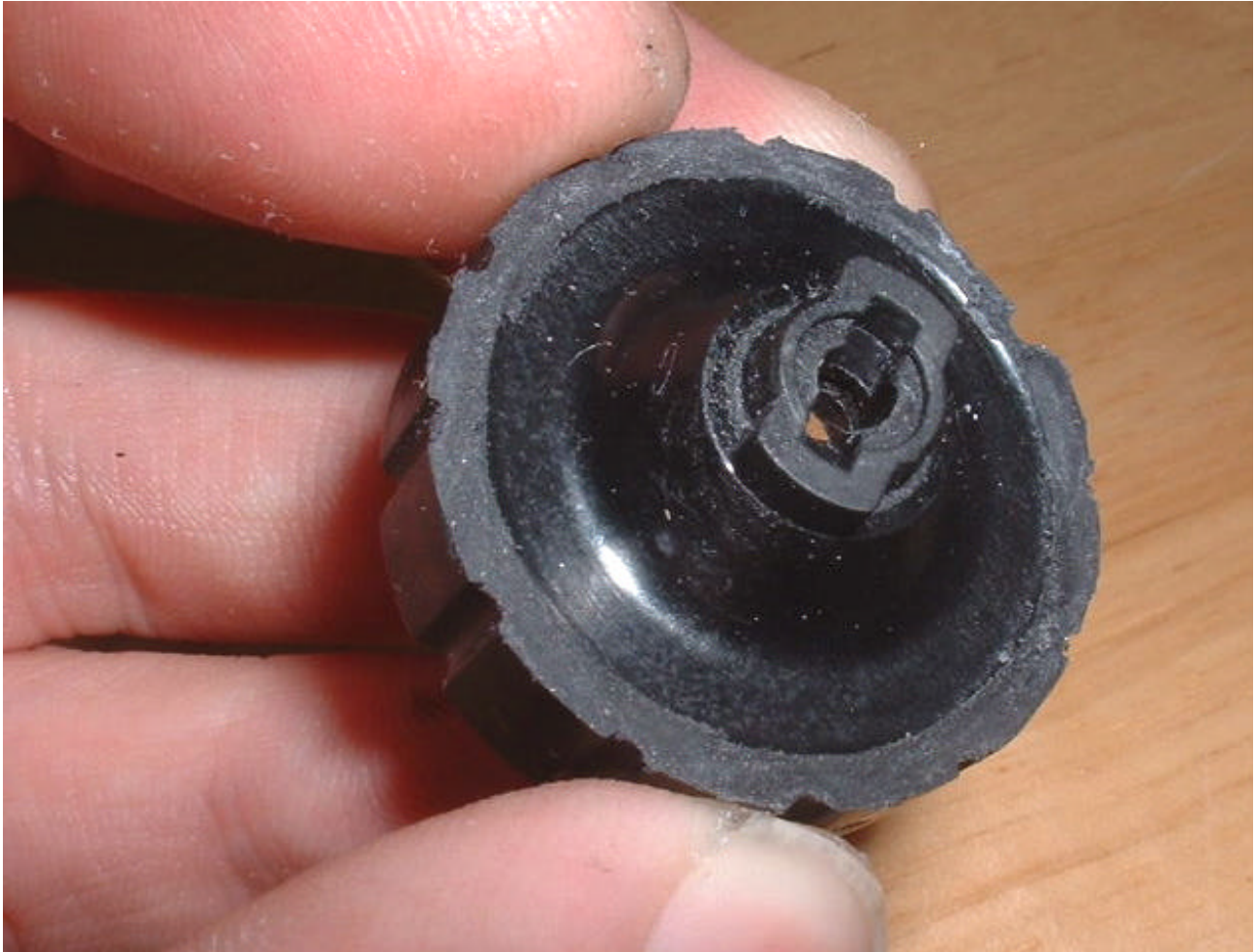
Figure 13. Finished inner wheel drum with inner portion cut away.
