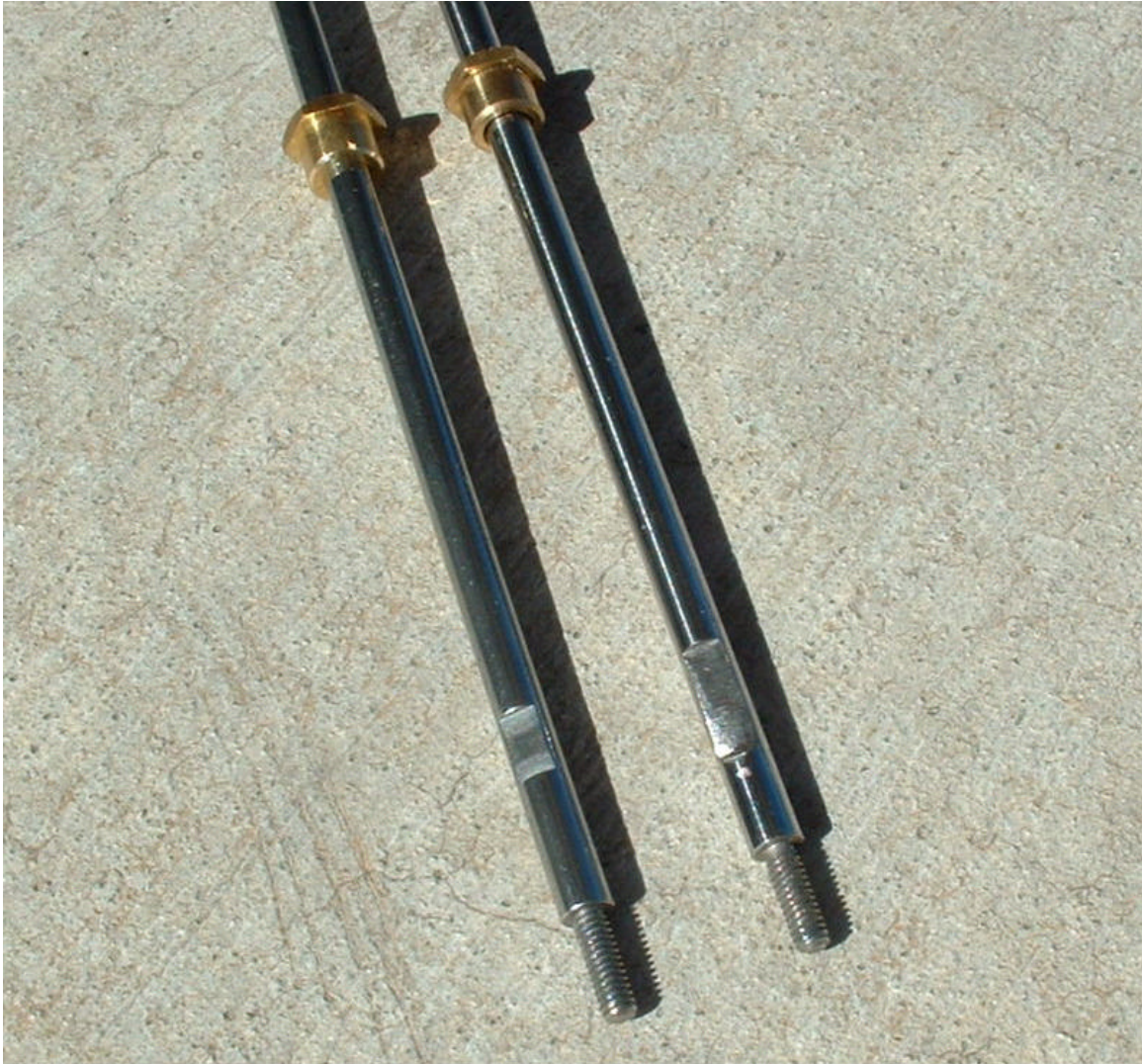
Figure 7. Lengthen the notch in the axle an extra 3mm.
