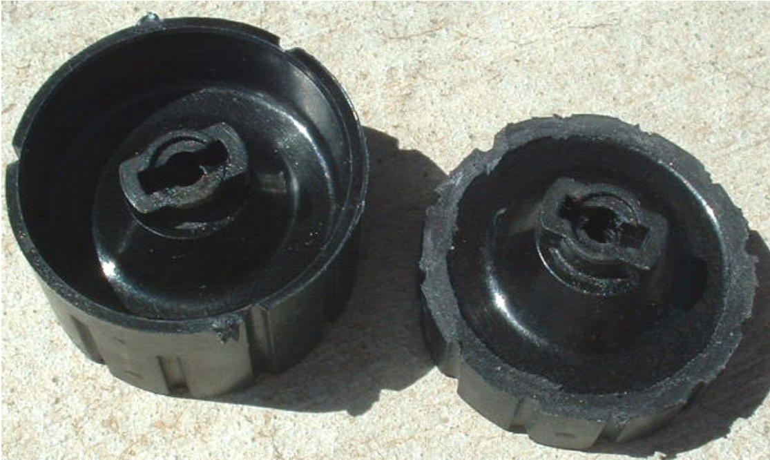
Figure 14. Comparison of a cut and uncut inner wheel drum.
