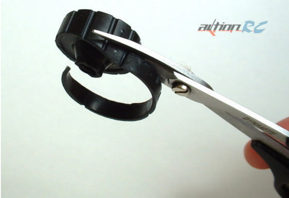
Figure 11. Cut from the outside edge to the center of the wheel drum and all the way around.
